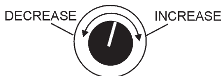
Figure 46. Voltage Adjust Control Knob
